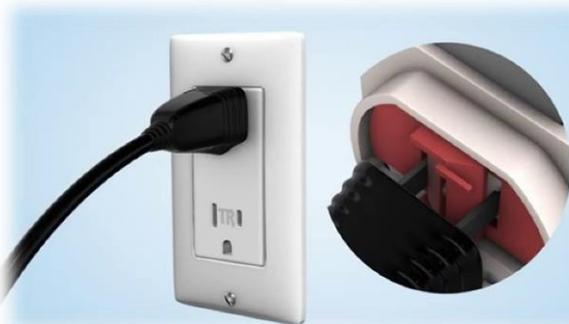
TRRs stands for Tamper Resistance Receptable. They provide a low maintenance solution to prevent childhood electrical shock and burns and now required in all new home construction. As stated from the Electrical Safety Foundation International, TRRs look just like ordinary outlets, but are designed with spring-loaded receptacle cover plates that close off the receptacle openings, or slots. When equal pressure is simultaneously applied to both sides, the receptacle cover plates open to allow the
